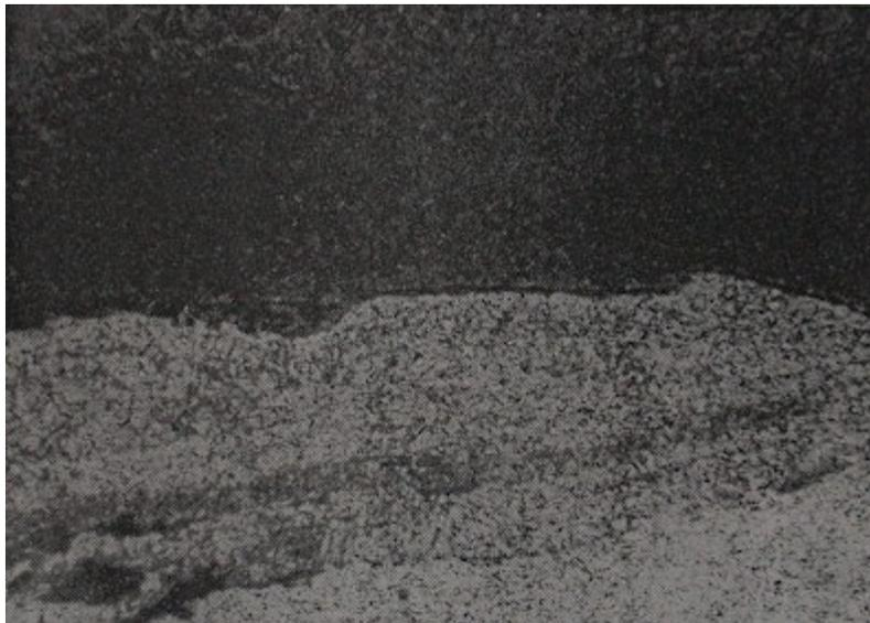
X 320. The decarburised area around the riveted joint. The low-carbon area is light-etching.
