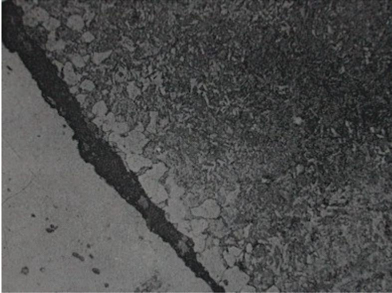
X 500. Martensite partly decarburised to ferrite at the joint
