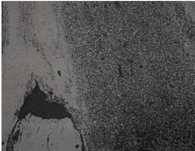
X 100. The area around the riveted joint.
